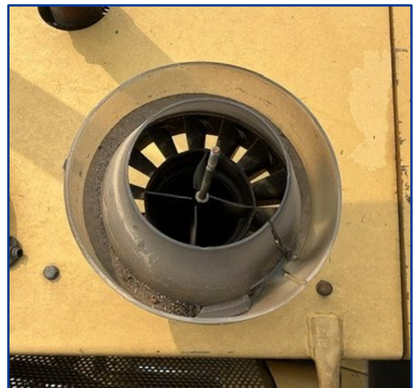
This photo shows the openings in the bottom of the pre-cleaner, where the embers likely entered the air filter.
